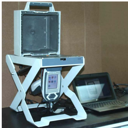
Figure 1. The handheld COTS XRF instrument used in the Heavy-Metal Paint Contamination project. The instrument is shown on the left, with the inset showing the built-in data display. The photo on the right shows the instrument mounted in its bench-top stand and connected to the laptop computer used to record and analyze the data.
